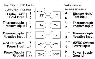
Pins (A,B) & (1,2) - Display Test/Display Hold Input: All numeric display segments will operate when Pins (A,B) & (1,2) are connected to +5VDC System Power Input Pins (H,J) & (7,8).
